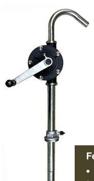
This is an advanced quality *Ryton Rotary Hand Pump* useful for most drums and tanks with a 2" Npt bunghole. Made from virgin grade oxidation resistant Ryton, Stainless Steel, PTFE and Buna-N (Nitrile or NBR). It can be mounted on 2" Npt bung holes of 15, 30, 55 gallon drums or bunged tanks.
