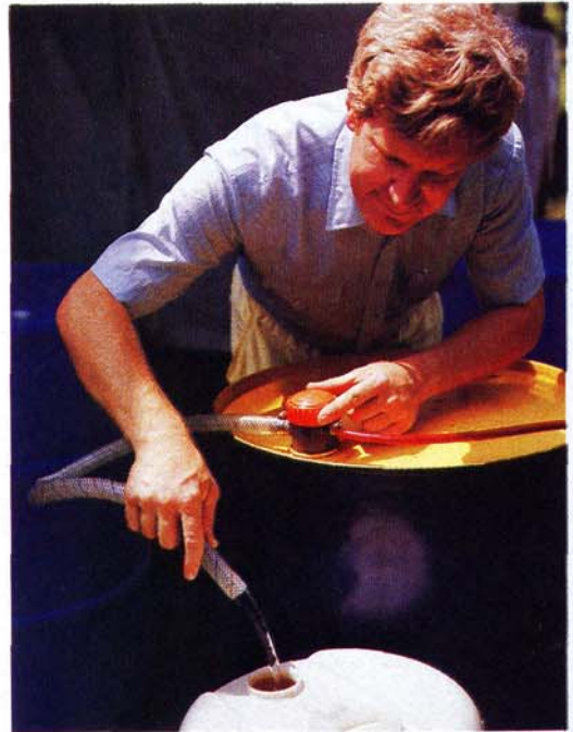
Drum pump dispenses hazardous liquids from steel drums used for storage and transport.
